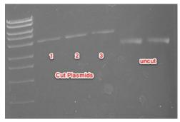
There is a noticeable difference between cut and uncut plasmids on gel. Next step is AP reaction.
