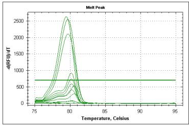
Above picture: Melt curve for VtpR primer set #4 (3 peaks). The other smaller peaks show the other primer sets not working as well.
